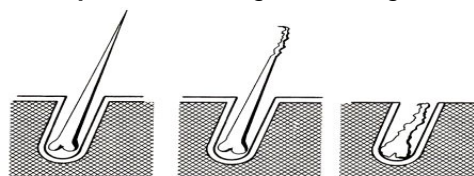
Fig. 1. Action of unhairing agent during \text{Na}_2\text{S} liming system sodium sulfide and sodium sulphhydrate used are sufficient
